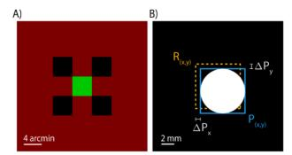
Fig. 1. TCA induced by pupil displacements. (A) The stimulus used for the alignment task. Subjects aligned a green ( $\lambda = 543$  nm) target square to be centered with respect to the surrounding decrement ( $\lambda = 840$  nm) squares. (B) Pupil tracking was performed in real time throughout the experiment. The experimenter induced pupil offsets relative to the reference pupil position,  $R_{(\alpha, \gamma)}$ .
