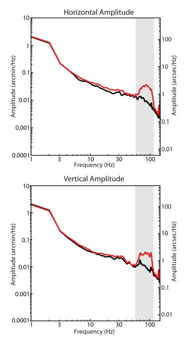
Figure 3. Amplitude spectra of an original AOSLO movie (black) and an AOSLO movie (red) that was digitally modified to include distortions from simulated tremor. The bump in the amplitude spectra from the modified AOSLO movie is clearly visible and matches the spectrum of the tremor that was digitally added.
