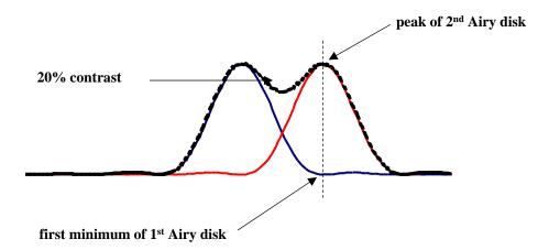
Recall that aberrations tend to blur ideal images. But even if there were no aberrations, rays would not be imaged to a point source but to a diffraction pattern. Perfect optical systems that have no aberrations are still limited by diffraction. A system that is free from aberrations is called **diffraction-limited** (ie its image quality is limited solely by diffraction)
