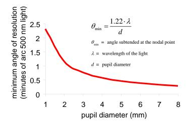
The graph plots the minimum angle separation that two point objects have to be separated by to be resolved in a diffraction-limited system. The smaller the minimum angle of resolution, the better the vision.
