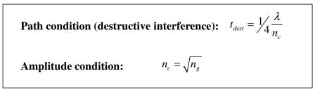
So, what are the problems with ARCs? They can make coatings of exact thicknesses, but the constraint is on available materials that meet the amplitude condition requirement.
