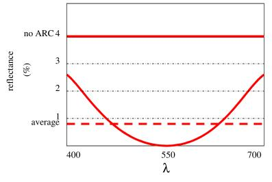
A typical ARC has an average of about 2% reflectance
