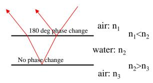
So the condition is opposite to that of an anti-reflection coating, because there is already a 180 deg phase difference between the two waves because one of the phases is not shifted. So, if the total path through the film is one half of a wavelength, then the light constructively interferes, not destructively as was the case for the ARC. Because the thickness of a soapy film constantly changes, you'll see a spectrum of different colors across the soap bubble.
