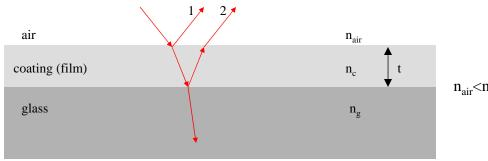
But there is a second condition that needs to be satisfied in order to maximize the amount of destructive interference. For complete destructive interference, we also require that the *amplitudes* of ray 1 and 2 be the same. To meet this requirement we need to have the condition that the reflectivity of the air coating interface and the coating glass interface be the same.
